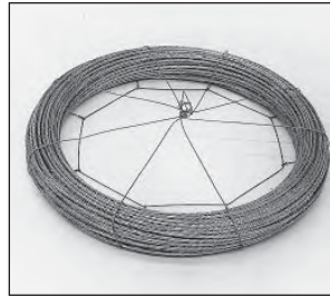
3. Twist at least two inches of legs together until wire cage is tight.
