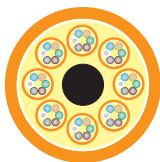
48-fibers (8 tubes of 6-fibers)
