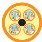
48-fibers (4 tubes of 12-fibers)
