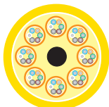
48-fibers (8 tubes of 6-fibers)
