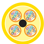
48-fibers (4 tubes of 12-fibers)
